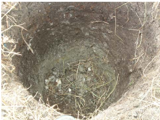
Plate 4: Trial hole in weathered S/S at Dartford site.
